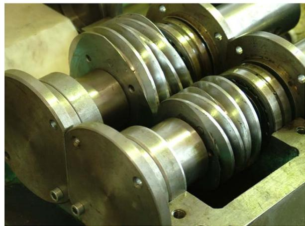
Figure 8. Helical gearing after test by loading 7<sup>th</sup> stage
