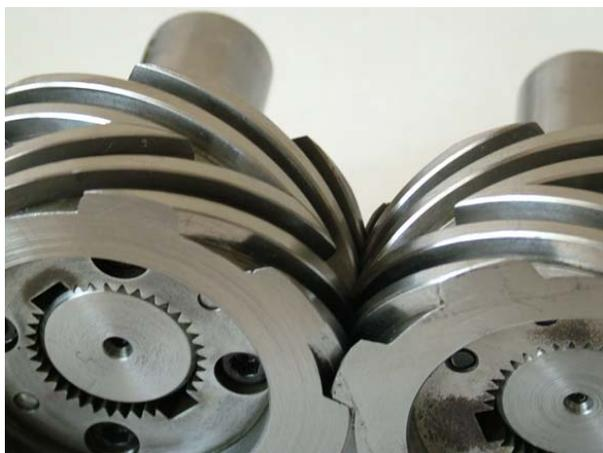
Figure 3. The screw gearing with parallel axes of rotation
