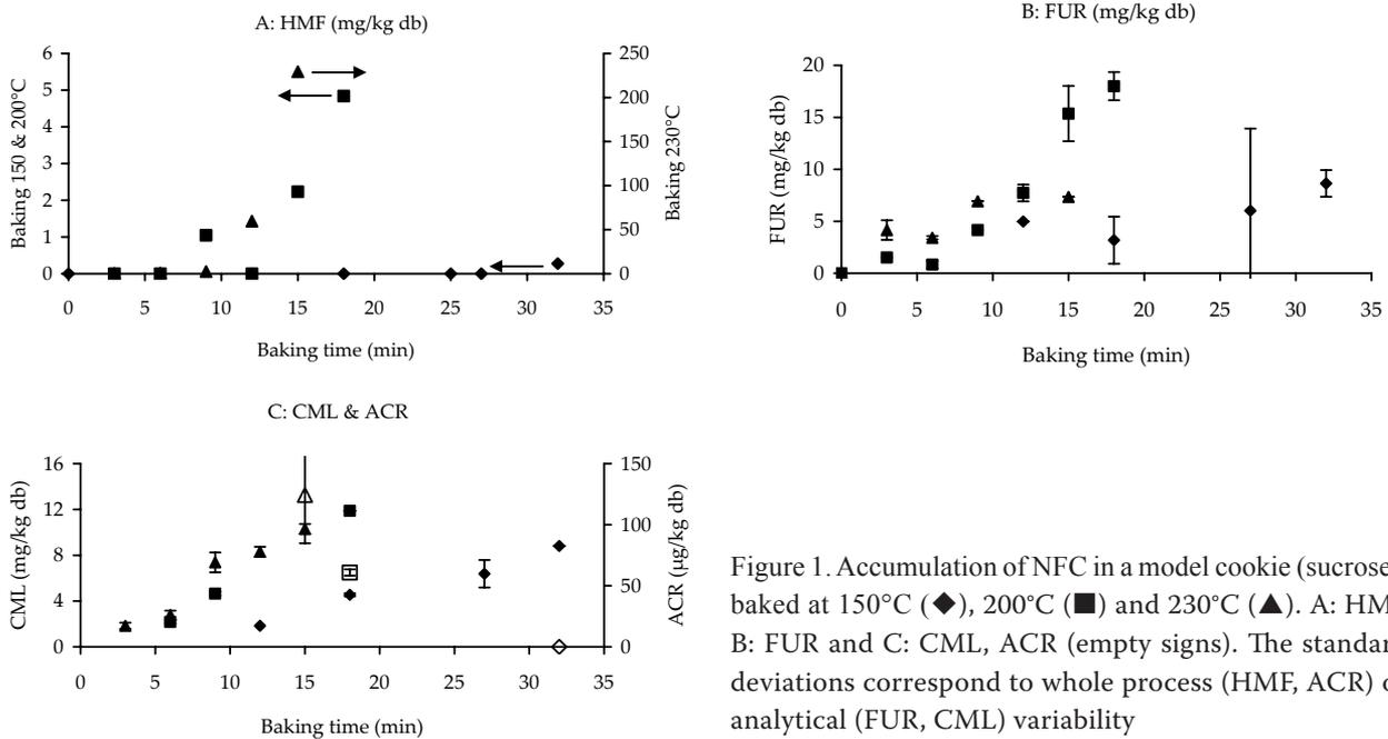
Figure 1. Accumulation of NFC in a model cookie (sucrose), baked at 150°C (◆), 200°C (■) and 230°C (▲). A: HMF B: FUR and C: CML, ACR (empty signs). The standard deviations correspond to whole process (HMF, ACR) or analytical (FUR, CML) variability
