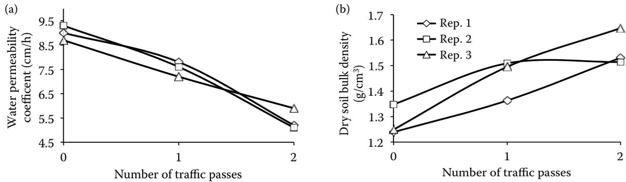
Fig. 2. Variation of average water permeability coefficient (a) and dry soil bulk density (b) as functions of the number of traffic passes
