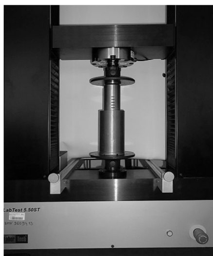
Fig. 2. Pressing of seeds and kernels of Jatropha curcas
