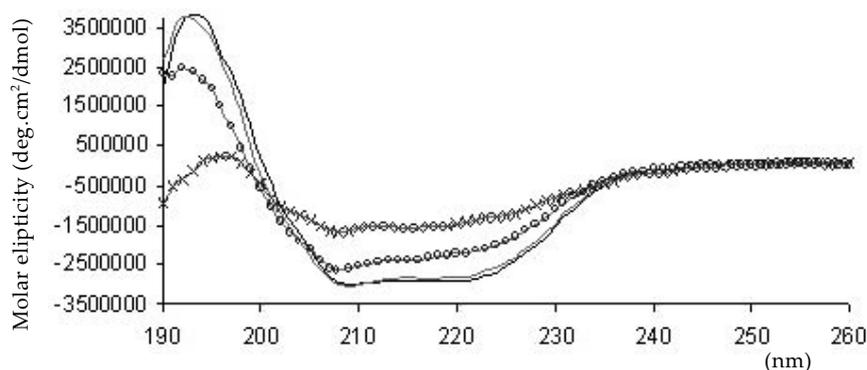
Figure 2. Far-UV CD spectra of MTG at different temperatures and pressures. Native (-), 400 MPa, 30 min at 40°C (--), 600 MPa, 60 min at 40°C (-o-), 80°C, 2 min (+++)
