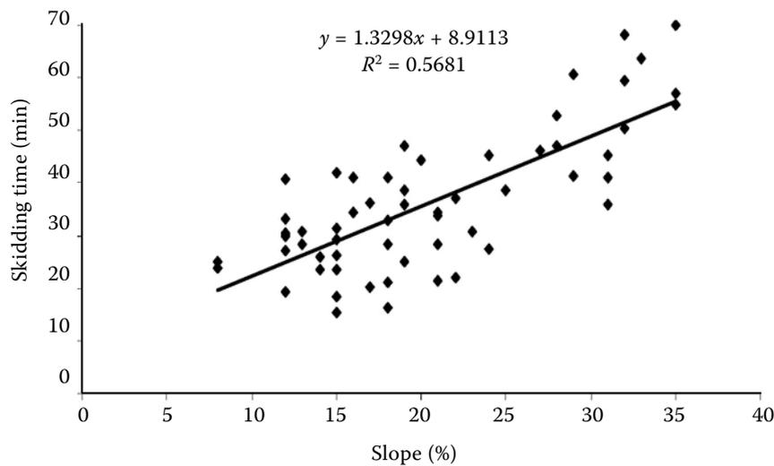
Fig. 2. Effect of slope on skidding time
