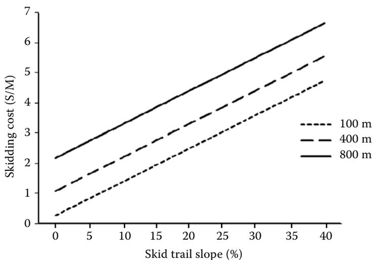
Fig. 3. Relative effect on cost as skid trail slope and skidding distance
