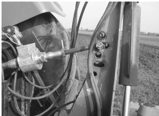
Fig. 1. Connection of top link with inserted load cell
