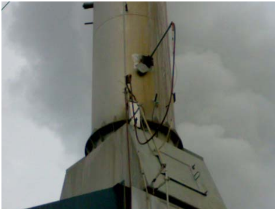
Fig. 6. Location of off-gas sampling probe in the stack thermo-oxidative equipment
