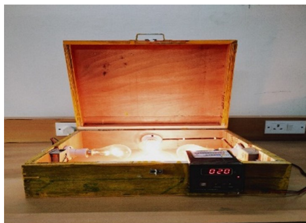
Figure 2. Temperature controller-sensor device for the temperature measurement
