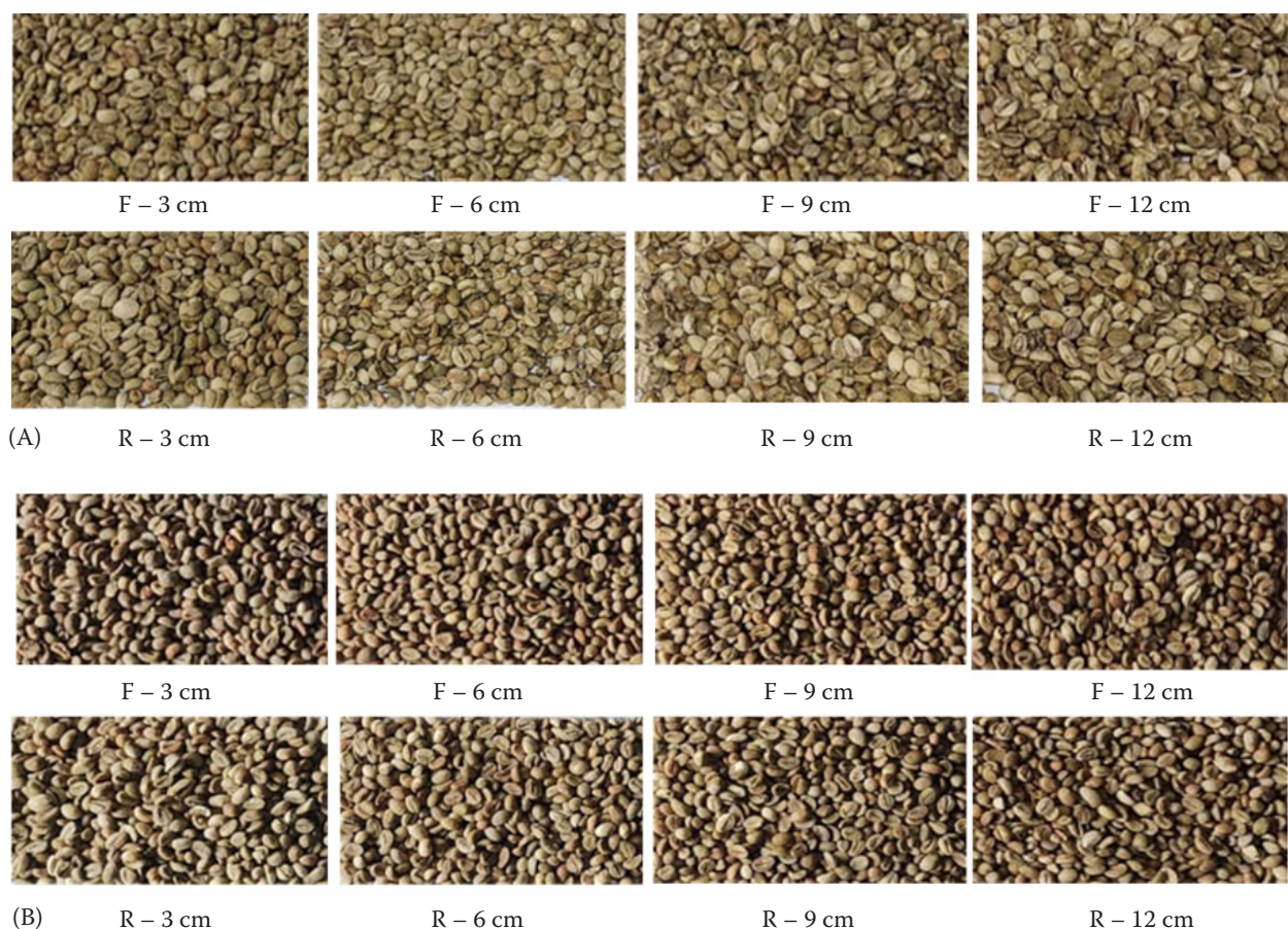
Figure 5. Coffee bean colour – (A) solar energy drying, (B) biomass energy drying F – front drying room; R – rear drying room, 3 cm to 12 cm bed thickness
