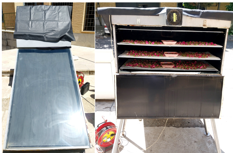
Figure 4. Indirect solar dryer for drying the Rosa flower buds
