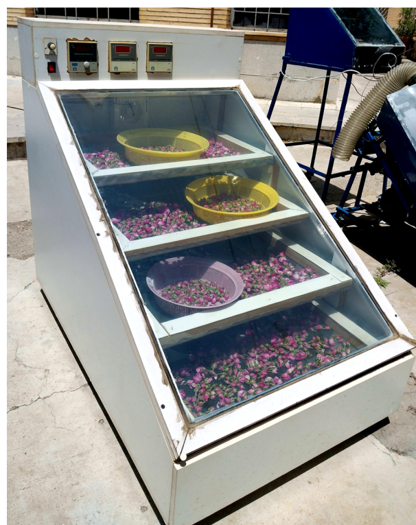
Figure 3. Direct solar dryer for drying the Rosa flower buds
