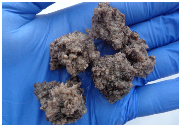
Figure 5. Five amorphous samples delivered to the laboratory, with numerous fine surface protrusions that easily broke off and crumbled into miniature pieces
