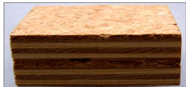
Fig. 3. Plywood with a cork core and a cork wear layer (12-ply, thickness 25 mm)
