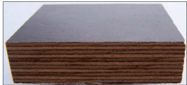
Fig. 1. Variant 1 – plywood with fibreglass (11-ply, thickness 16 mm)
