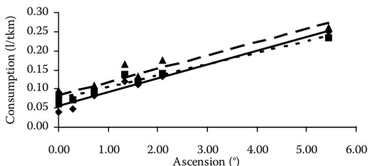
Figure 7. Dependence of the specific fuel consumption (l/tkm) on the driving route ascension when transporting load with the 5.8 t mass
