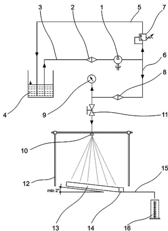
Figure 3. Scheme of the device for water surface runoff with volume reading in calibrating cylinder
