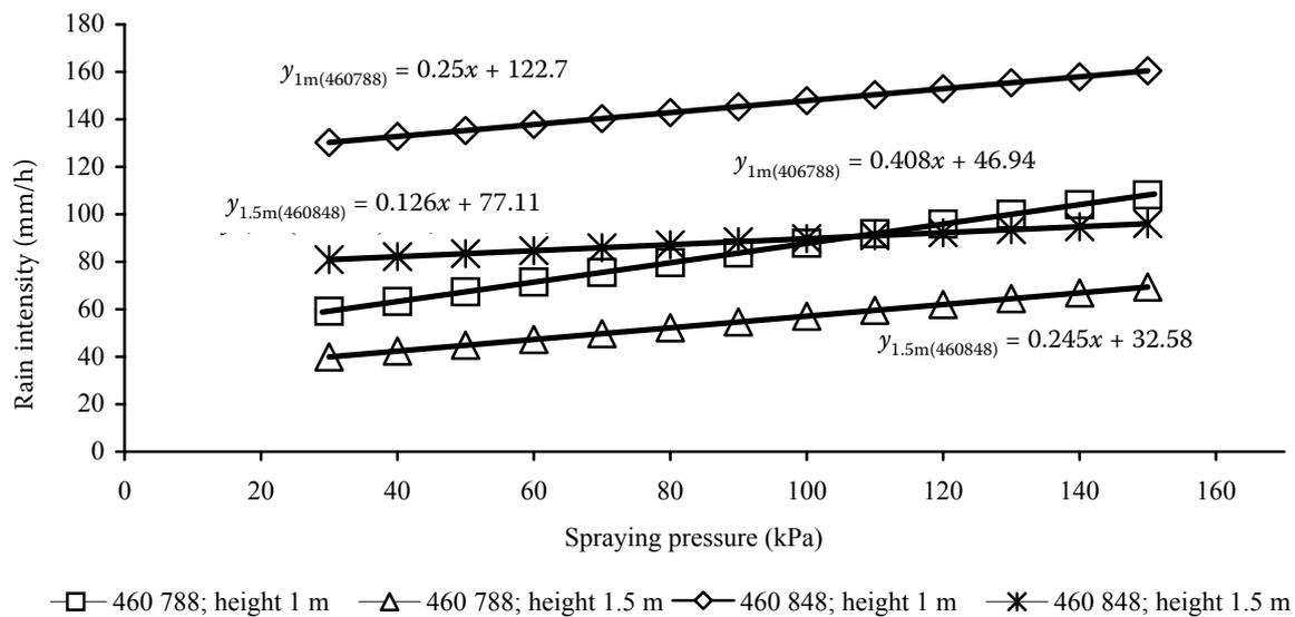
Figure 1. Calibration straight lines of simulated rain intensity per measuring surface of  $0.7 \times 0.7$  m for nozzles Lechler 460 788 and 460 848 in dependence on adjustable spraying pressure and height
