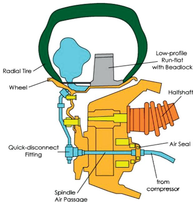
Fig. 1. Central Tire Inflation System at the wheel (Lynch Hummer 2006)
