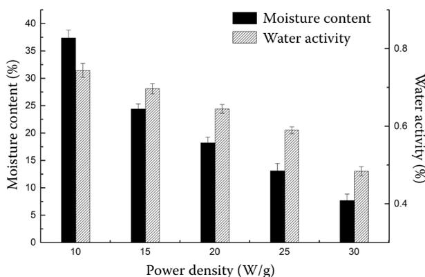
Figure 5. Effect of power density on moisture change of tilapia fillets after osmotically dehydrated vacuum-microwave drying (OD-VMD)
