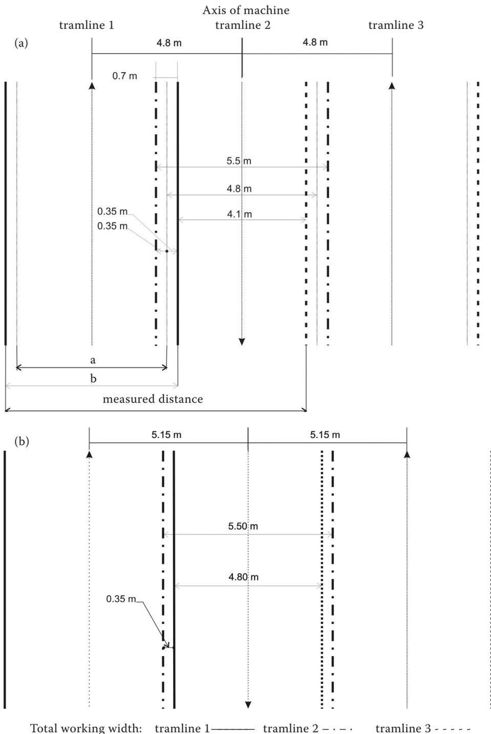
Fig. 2. Scheme of machine tramlines for navigation at (a) 4.8 m and (b) at 5.15 m
