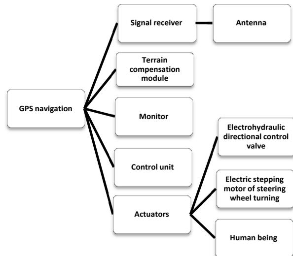
Fig. 1. Navigation system elements where failures are possible to occur
