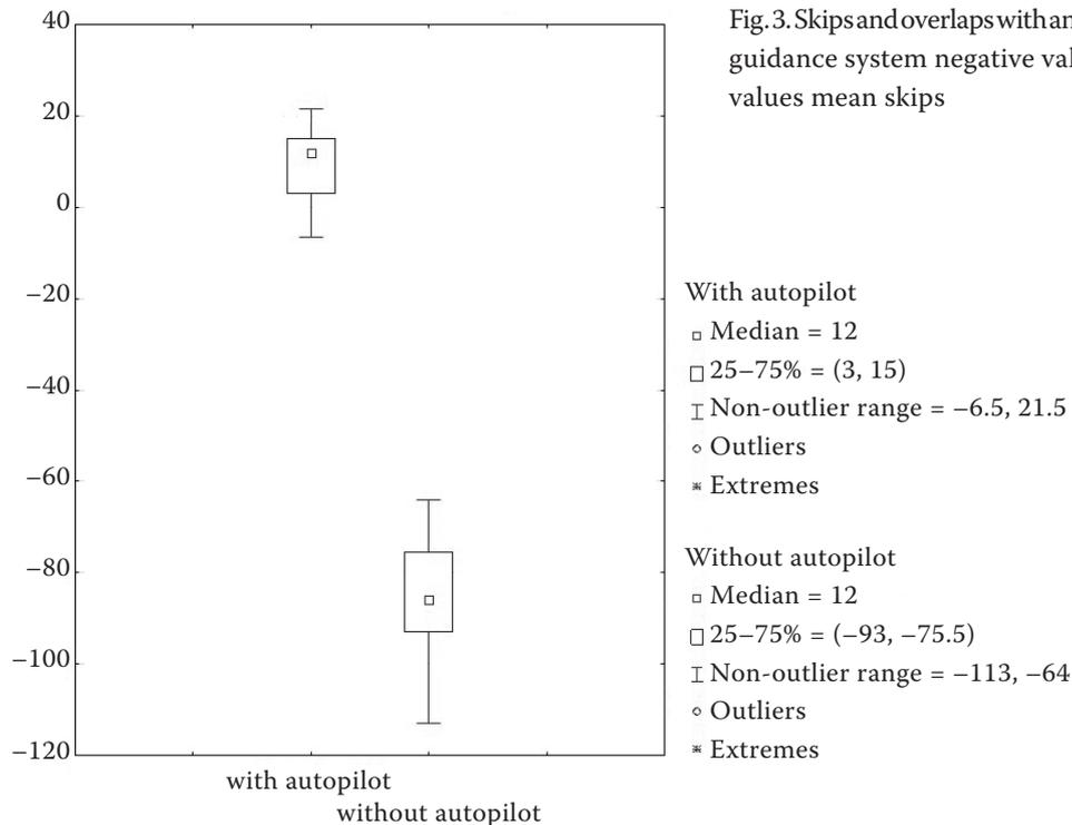
of agronomical requirements on tillage. An unnecessary large overlap occurred due to setting an incorrect value of working width for the satellite navigation system. Based on such experiments and failures recorded by machine operators and service workers, we determined the risks associated with using satellite navigation systems.
