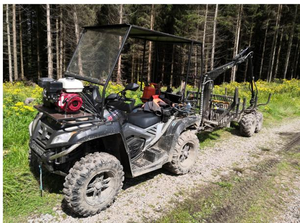
Figure 1. ATV Forwarder – CF Moto Gladiator V800 EFI ATV and Vahva Jussi 1500/320
