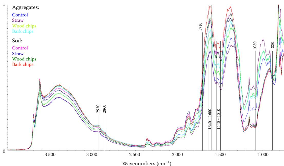
Figure 1. Average diffuse reflectance infrared spectroscopy with Fourier transformation (DRIFT) spectra of studied treatments normalized to the maximum intensity (800/ $\text{cm}$ )
