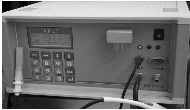
Fig. 4. Equipment for biogas analysing (analyser AIR LF)
