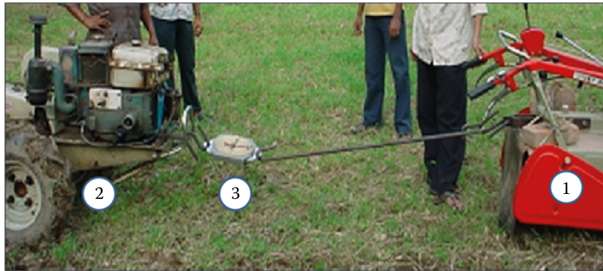
Figure 1. Test set-up for the power tiller's drawbar performance evaluation
