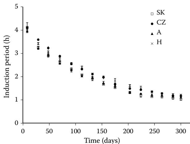
Figure 1. Oxidative stability of investigated sunflower oils expressed as induction periods determined by the Rancimat test under accelerated conditions (110°C, 20 l/h air flow)
