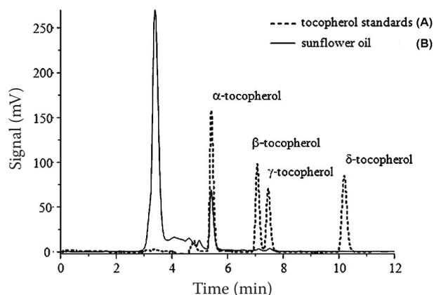
Figure 2. Determination of individual tocopherols by HPLC: (A) chromatogram of individual tocopherols determined in a model mixture composed of tocopherol standards and (B) chromatogram of individual tocopherols naturally present in the sample of initial sunflower oil (SK) used in the storage experiment
