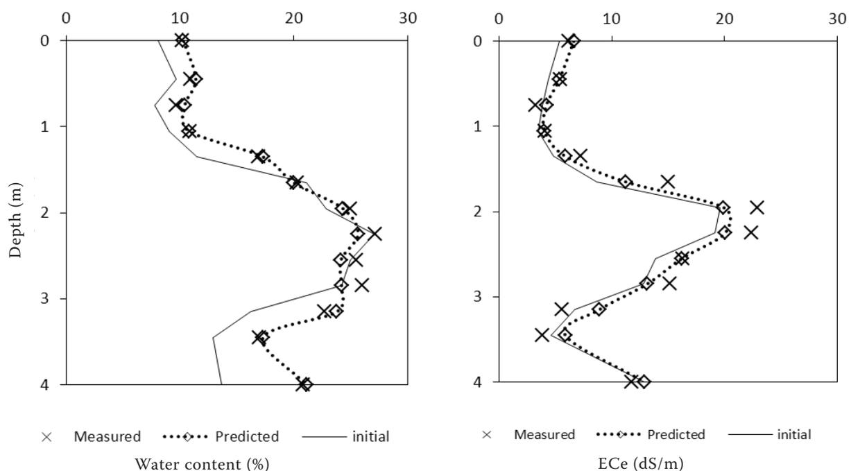
Figure 1. Measured and predicted profiles of 10<sup>th</sup> day of flood irrigation experiment
