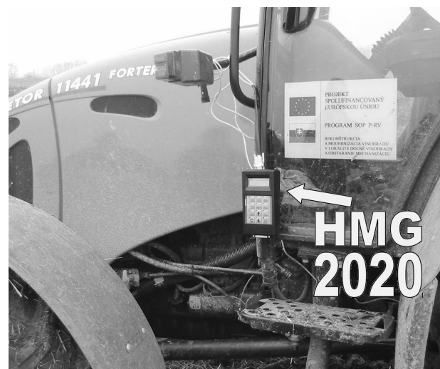
Fig. 3. Fluid temperature measurement under operating conditions
