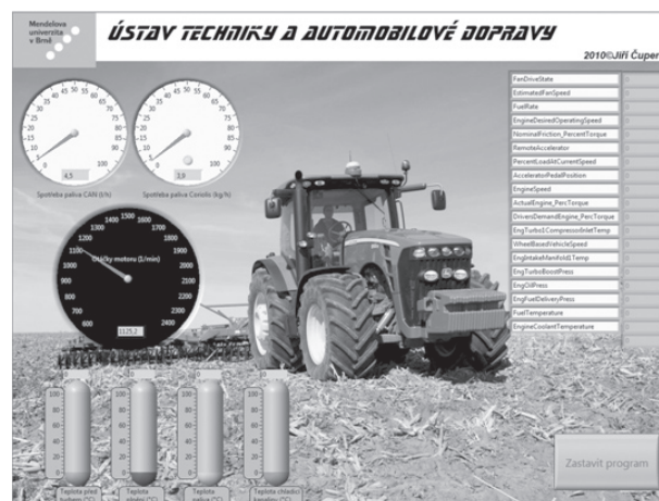
Fig. 3. Front panel of the software used for CAN listening
