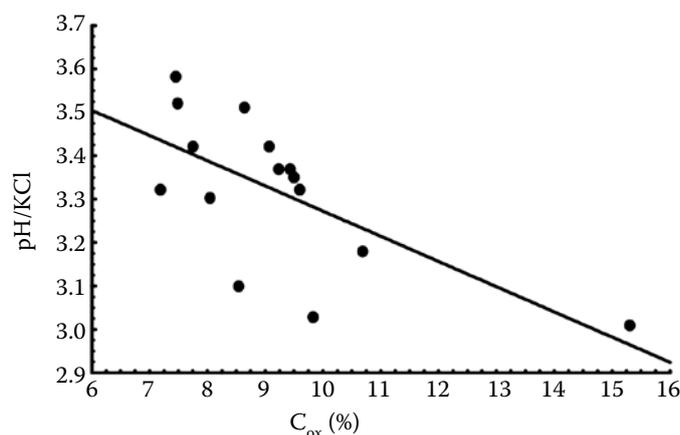
Fig. 5. Linear regression of  $C_{ox}$  and pH/KCl in Suchdol locality
