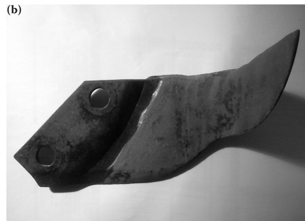
Fig. 5. Application example: (a) rotary tiller blades and (b) blade with composite
