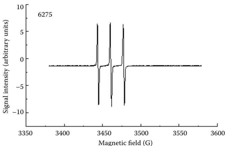
Figure 1. EPR spectrum of stable radical Tempol (2,2,6,6-tetramethylpiperidine-1-oxyl) (aqueous solution), temperature 25°C
