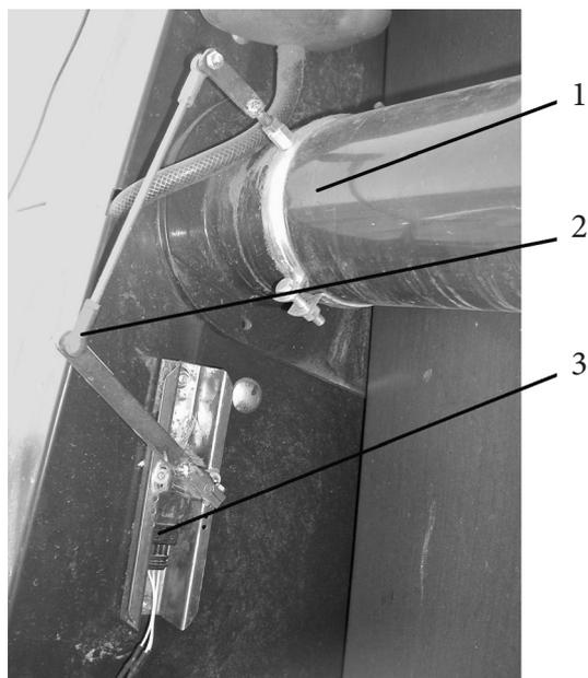
Fig. 1. Technical description of potentiometer position
