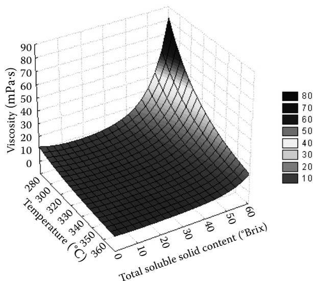
Figure 2. Surface plot for combined effect of temperature and total soluble solid content on viscosity of enzyme clarified lime juice
