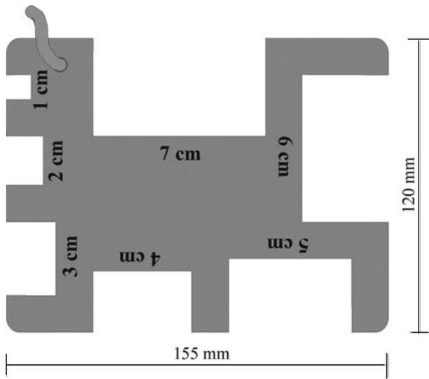
Fig. 3. Simple measuring tool used for measuring diameter of small-sized wood
