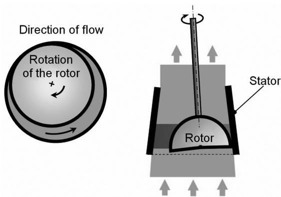
Figure 1. Principle of bladeless turbine (POLÁK *et al.* 2013)
