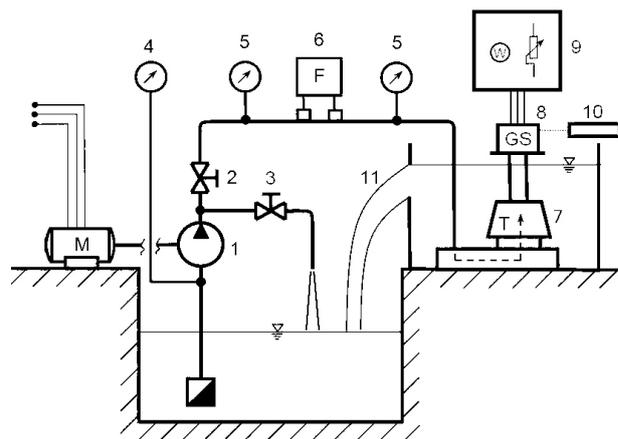
Figure 3. Diagram of the hydraulic circuit for measuring the DVE 120 miniturbine (DLABAL *et al.* 2015)
