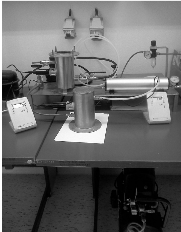
Fig. 4. Equipment of measurement of gas permeability
