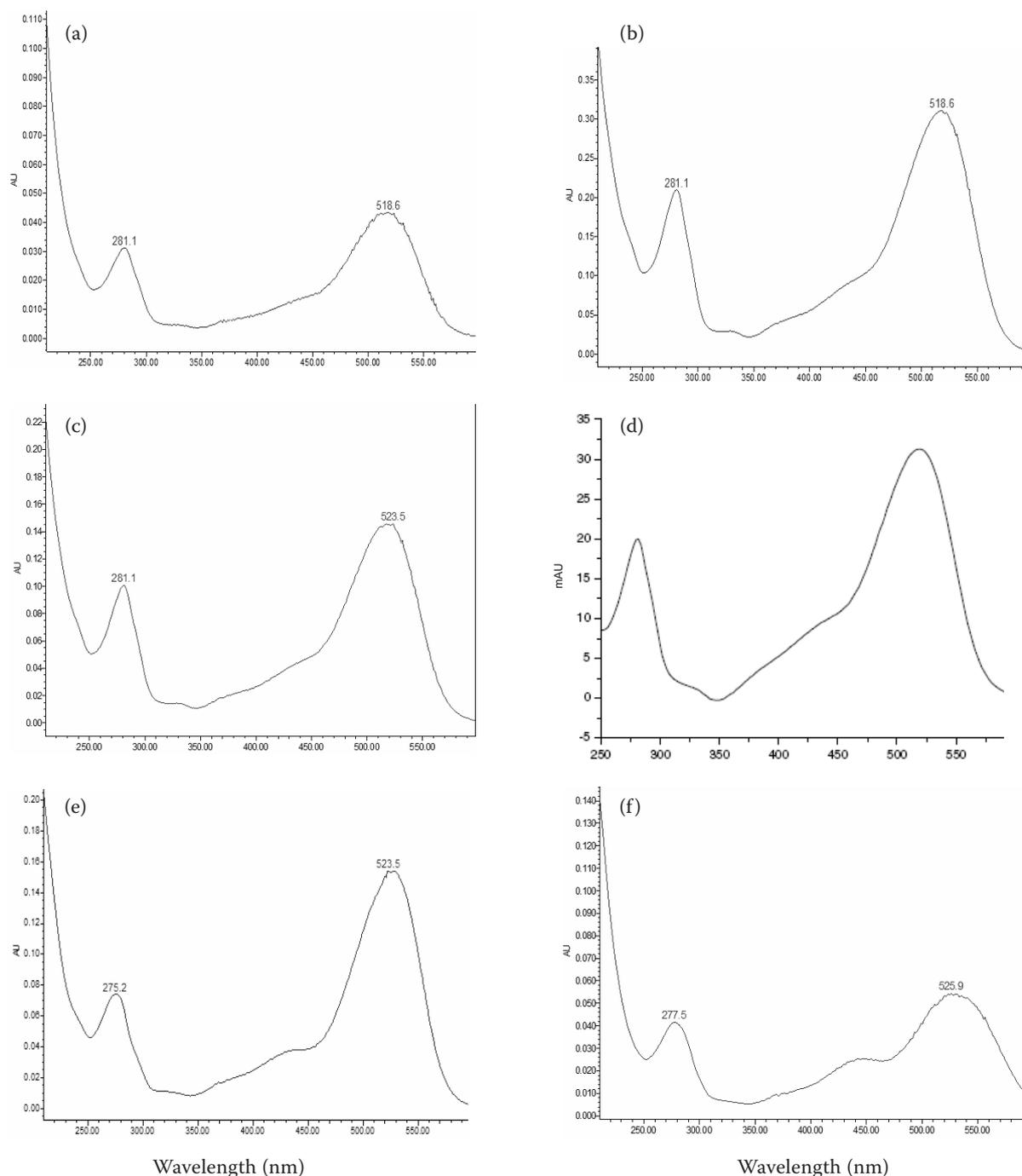
Figure 5. UV-Visible spectrum of peaks 1–5 recorded with a photodiode array detector (PAD) from 200 nm to 600 nm: (a) peak 1; (b) peak 2; (c) peak 3; (d) standard cyanidin 3-*O*-glucoside (Cy-3-Glu); (e) peak 4; (f) peak 5
