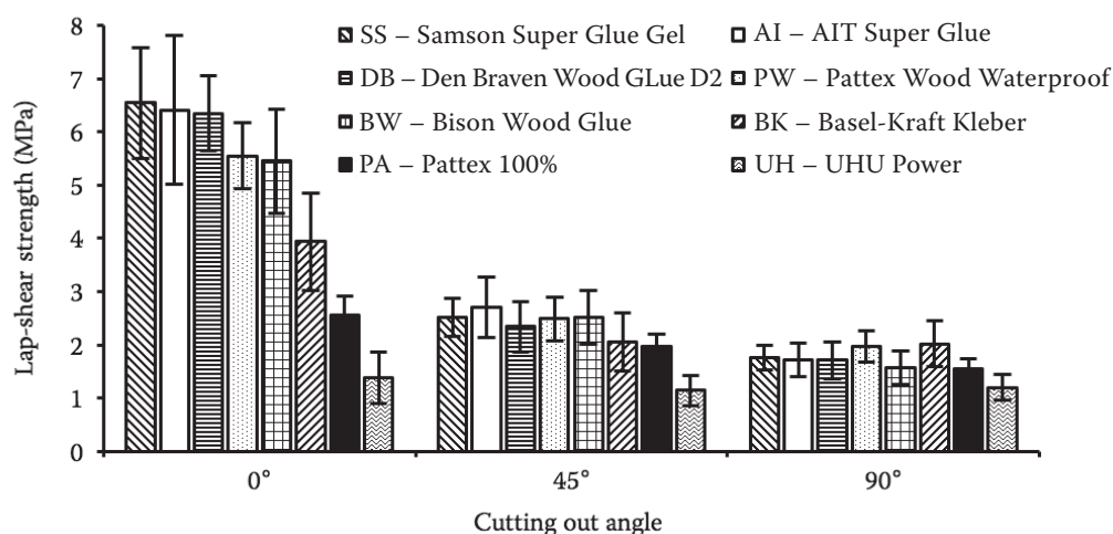
Fig. 2. Relationship between the tensile lap-shear strength and the cutting out angle; standard
