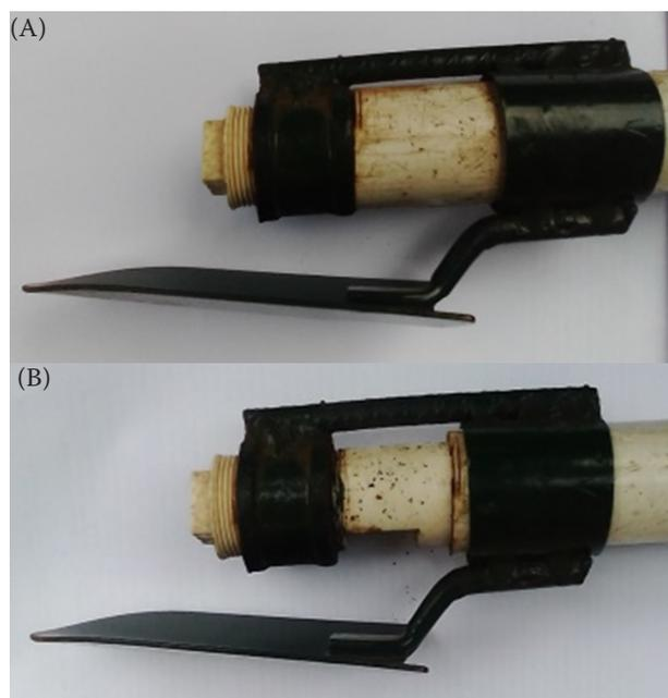
Figure 2. Discharge chute (A) closed and (B) open
