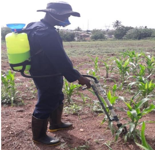
Figure 3. Manual fertiliser applicator in operation
