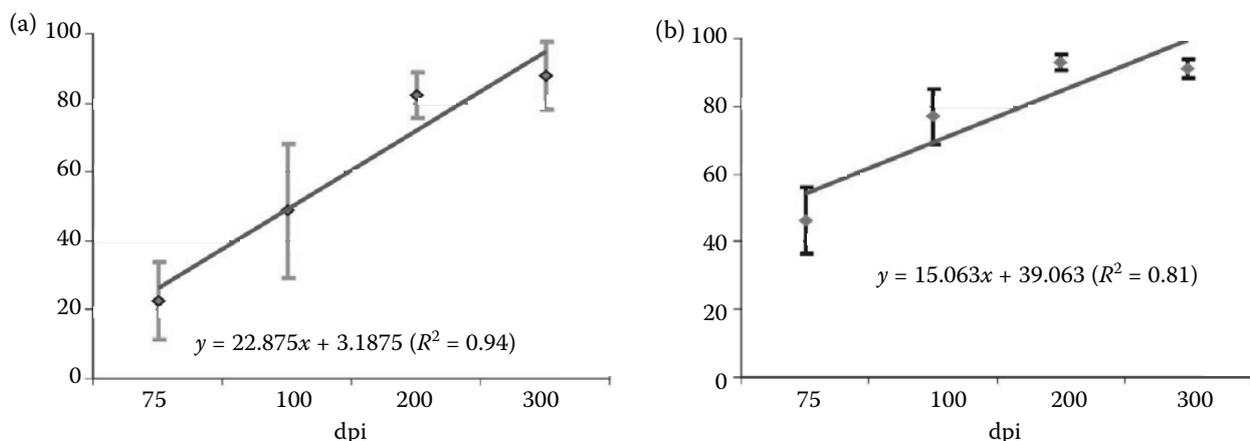
Figure 5. Accuracy of automatic procedure of image analysis (%) for each scanning resolution of roentgenograms of cracked (a), and infested (b) kernels
