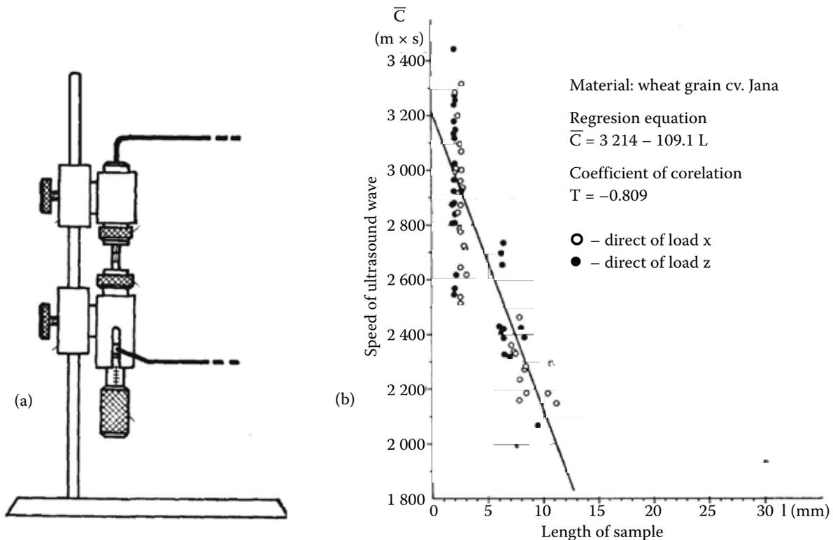
Figure 4. Diagram of the mechanical part of the equipment used to measure the speed of ultrasound waves in grain endosperm (a), and the values of the speed of ultrasound wave front in the endosperm of wheat and the course of its regression dependence on the height of sample column (b)
