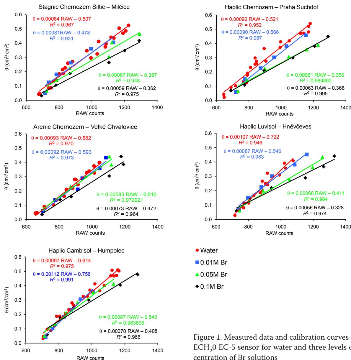
Figure 1. Measured data and calibration curves for the ECH<sub>2</sub>O EC-5 sensor for water and three levels of concentration of Br solutions
