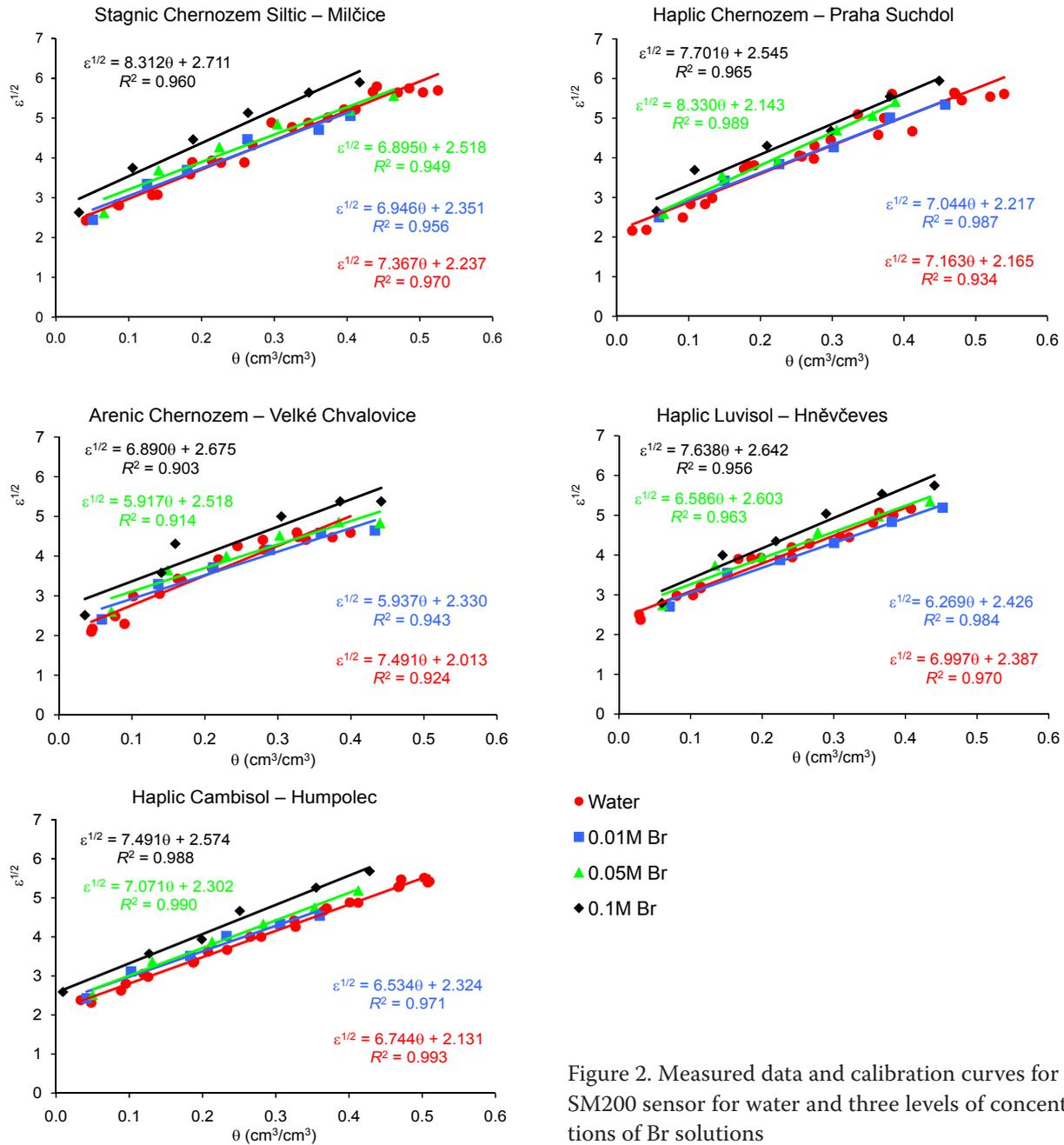
Figure 2. Measured data and calibration curves for the SM200 sensor for water and three levels of concentrations of Br solutions
