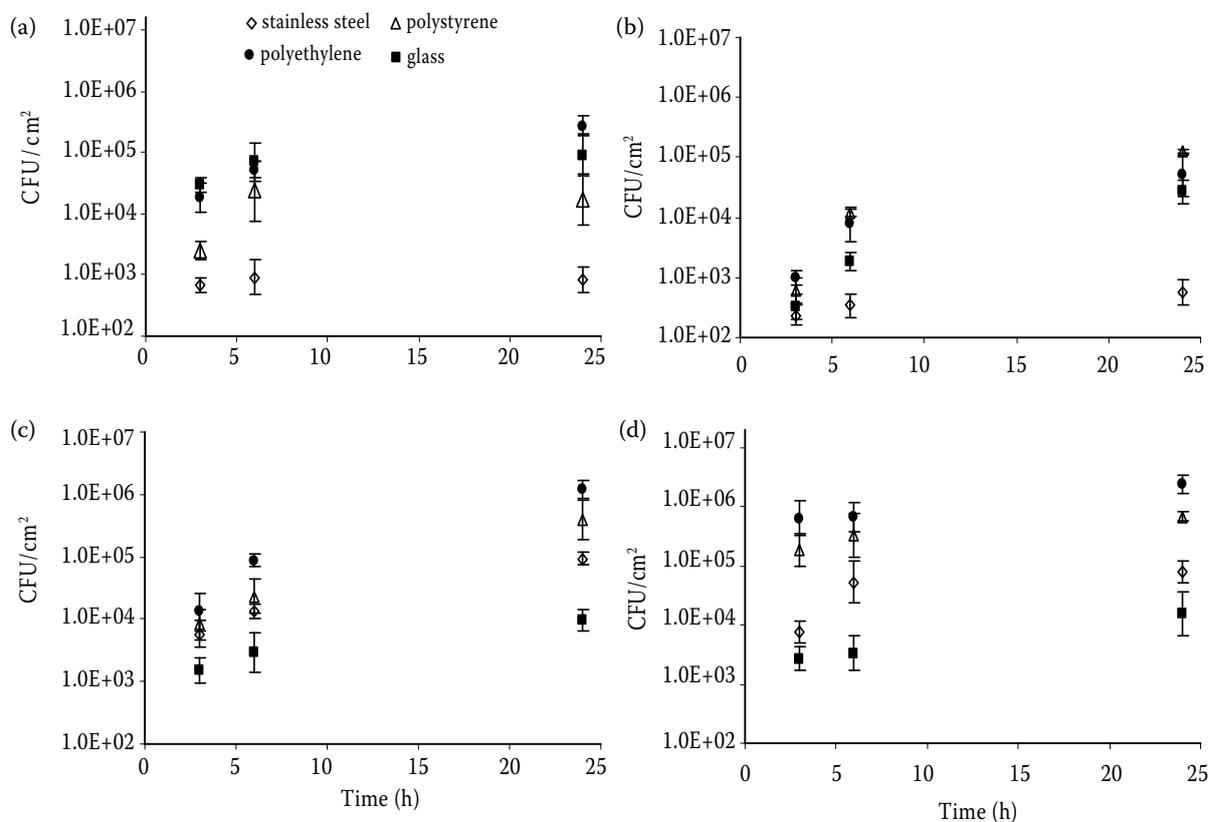
Figure 3. The bacterial adhesion of *A. bogorensis* (a), *E. coli* (b), *P. fluorescens* (c), and *Acinetobacter* spp. (ad to stainless steel, glass, polystyrene and polyethylene). The results are expressed as CFU/cm<sup>2</sup> after 3, 6 and 24 h incubation at the 25°C (*A. bogorensis*) and 37°C (the other tested microorganisms)
