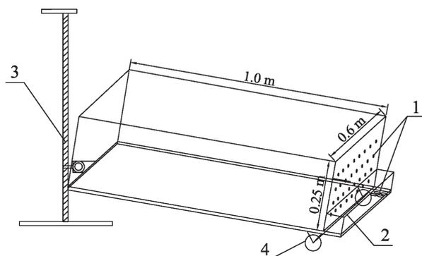
Figure 1. The structure of the soil groove (Ding et al. 2017)
