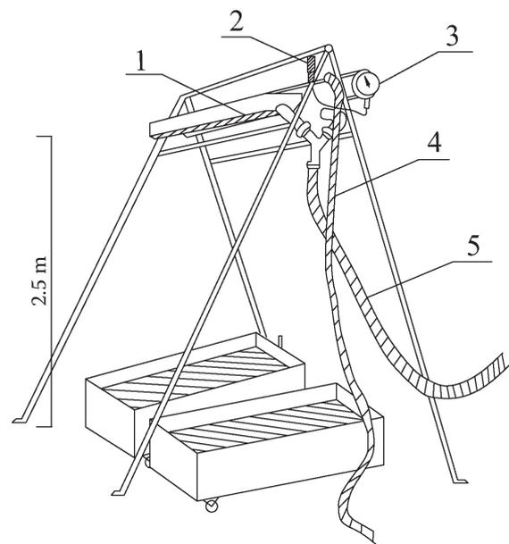
Figure 2. The structure of the NORTON artificial rainfall simulator (Ding et al. 2017)
