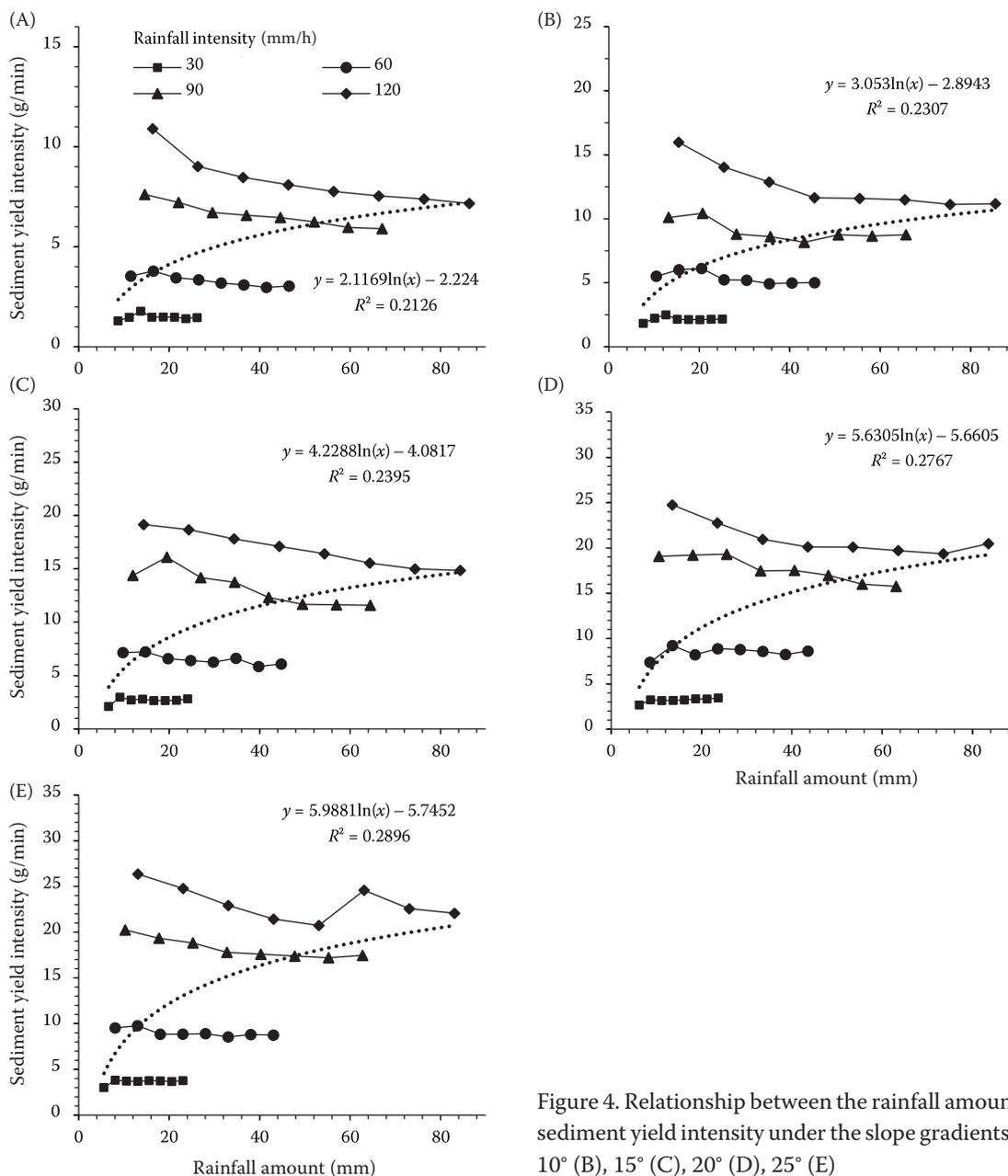
Figure 4. Relationship between the rainfall amount and the sediment yield intensity under the slope gradients of 5° (A), 10° (B), 15° (C), 20° (D), 25° (E)
