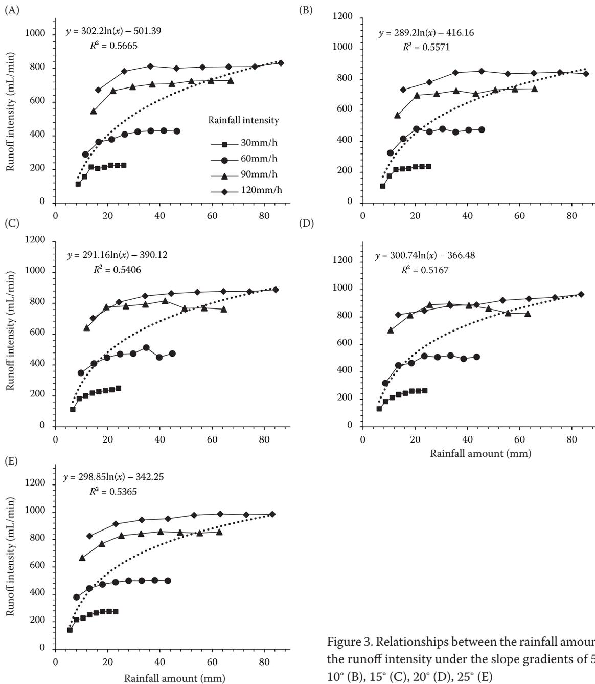
Figure 3. Relationships between the rainfall amount and the runoff intensity under the slope gradients of 5° (A), 10° (B), 15° (C), 20° (D), 25° (E)
