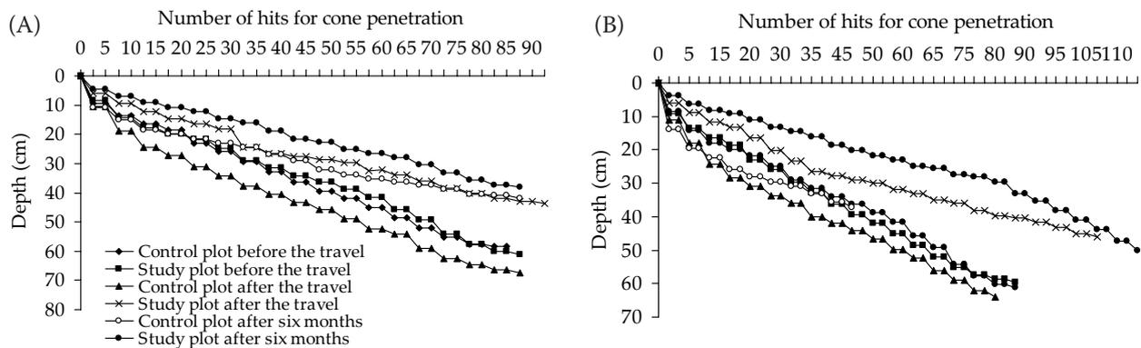
Fig. 3. Penetration curves on study plot No. 4, Rudice, Zetor 7245 universal wheeled tractor, three sets of measurements – (A) the first set and (B) the second set of measurement
