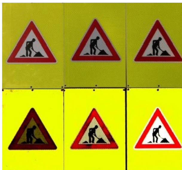
Figure 2. Combination of retroreflective sheeting on the "Work" traffic sign on a fluorescent substrate
