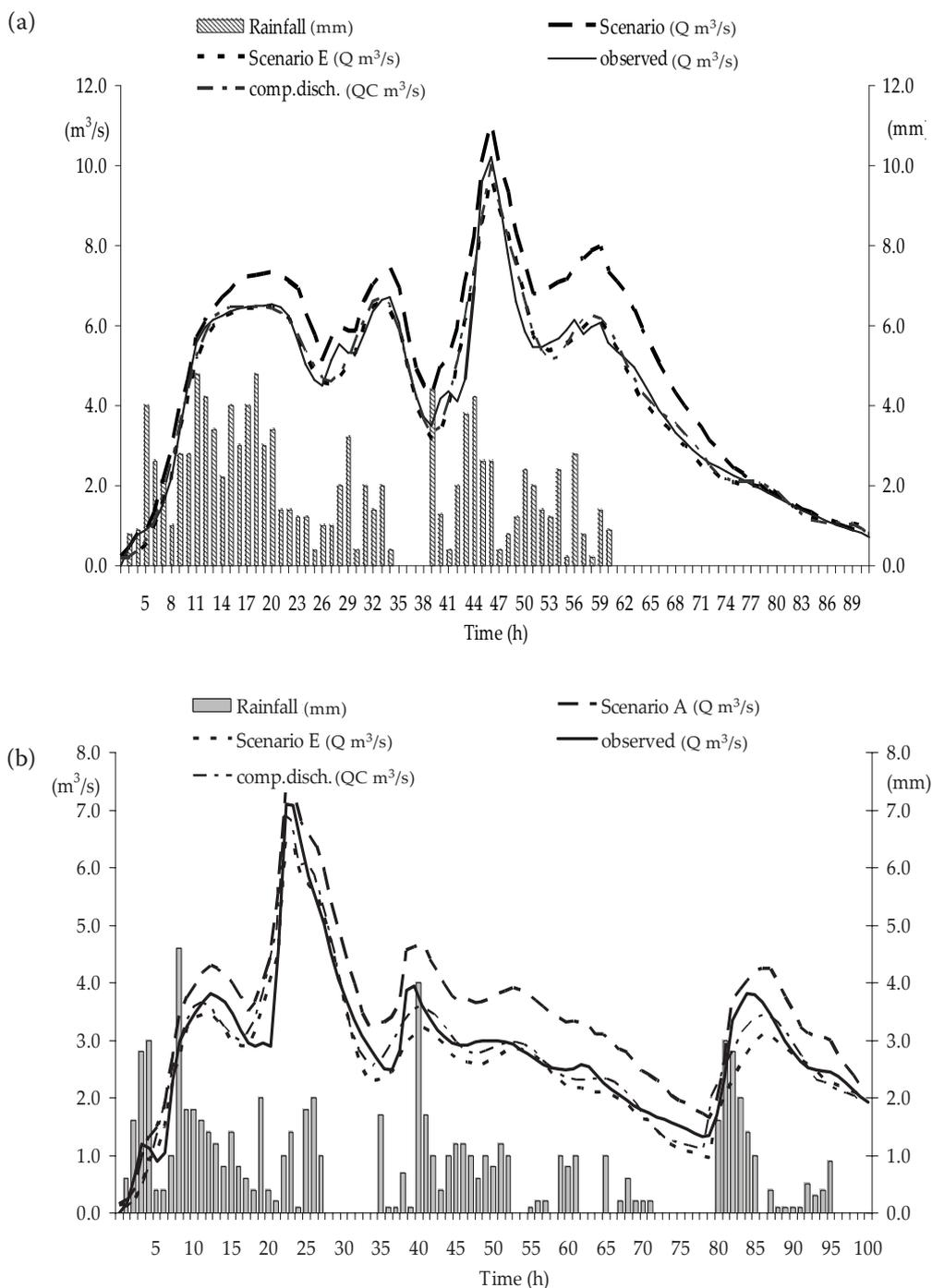
Figure 2. Comparison of ordinates of observed and reconstructed discharges (including scenarios) on the Všeminka catchment
