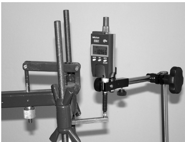
Fig. 1. Instrument for the measuring of eggshell deflection
