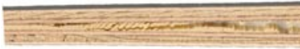
Fig. 30. Failure in the central zone due to shear stress in a combined plywood 18 mm thick
