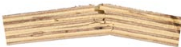
Fig. 26. Fibrous fracture along the height of the specimen in a combined plywood 18 mm thick
