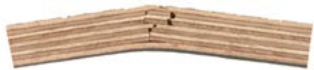
Fig. 27. Fibrous fracture along the height of the specimen in a beech plywood 15 mm thick
