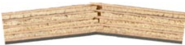
Fig. 25. Fracture along the height of the specimen in a combined plywood 18 mm thick
