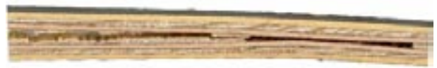
Fig. 31. Failure in the central zone due to shear stress caused by the defect of a central veneer in a combined plywood 10 mm thick
