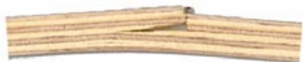
Fig. 28. Rupture of fibres in the tensile zone of the specimen in a combined plywood 15 mm thick
