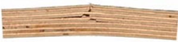
Fig. 29. Rupture of fibres in the tensile zone of the specimen in a beech plywood 18 mm thick
