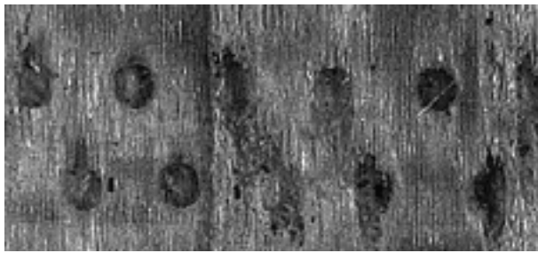
Fig. 1. Photo of penetration traces on the tested sample surface. Fine structure in the figure represents individual wood cells (tracheids). There is an order difference between diameters of the indenter and the individual tracheids
