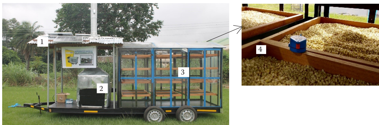
Figure 1. Developed mobile solar biomass hybrid dryer with Solar PV system 1 – solar PV system; 2 – furnace with enclosed heat exchanger and chimney; 3 – drying chamber with drying racks; 4 – insert of trays with maize in the dryer and logging device
