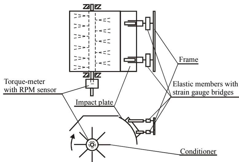
Fig. 1. Equipment for material feed rate measurement
