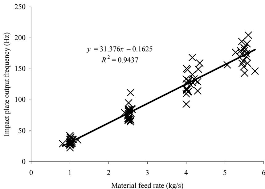
Fig. 4. Measured values from impact plate measurement
