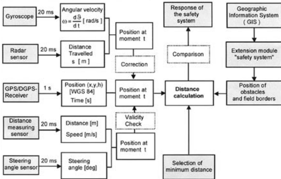
Fig. 2. Data flow in the safety system
