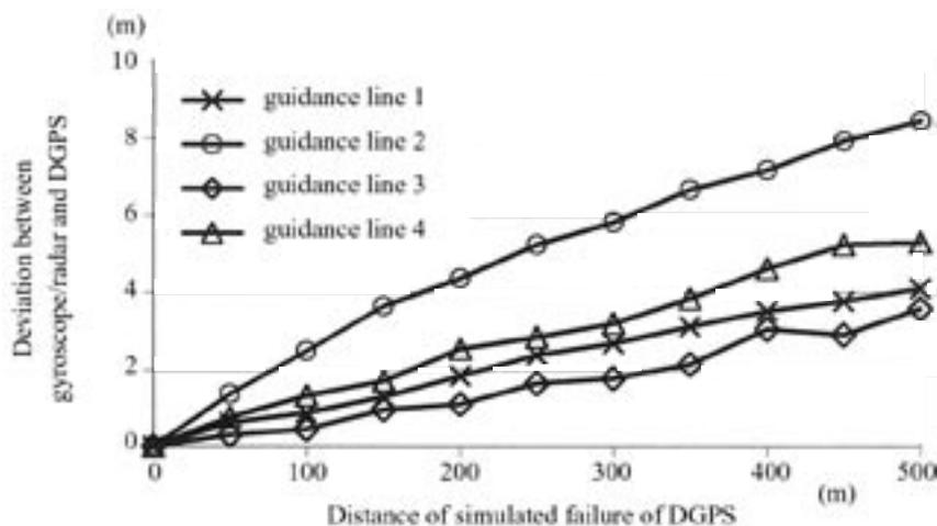
Fig. 5. Dependence of deviation between gyroscope/radar and DGPS on the distance
